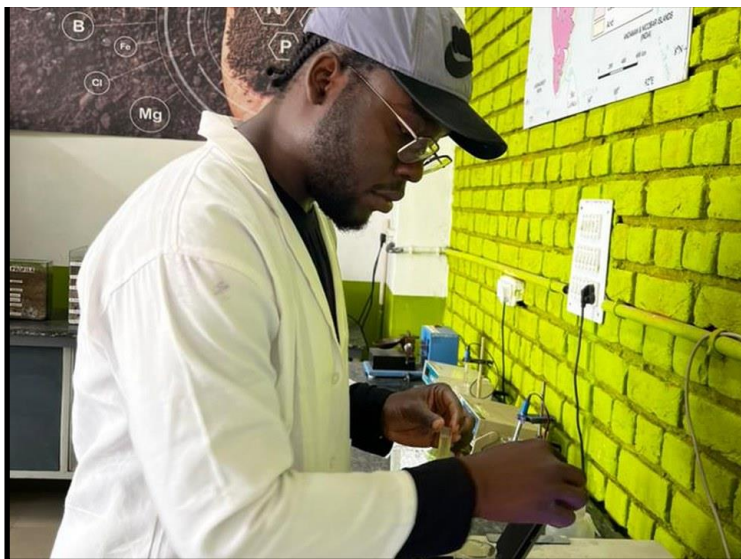
Figure 26: Determination of Phosphorus Content Using Spectrophotometric Method — LPU Laboratory
