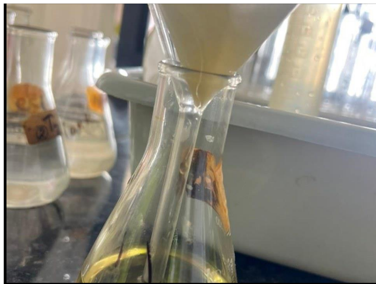
Figure 25: Filtration of Digested Sample During Chemical Analysis — LPU Laboratory
