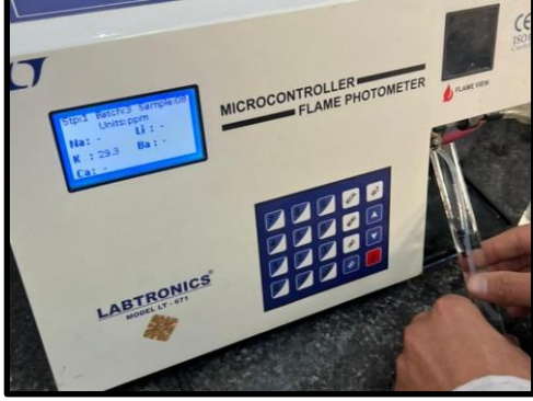
Figure 27: Determination of Potassium Content by Flame Photometer (Labtronics LT-671) — LPU Laboratory
